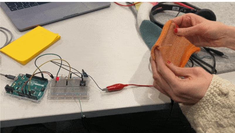
These sensors can be used anywhere a potentiometer would be used instead. Typically the signal is much noisier and harder to control, but you can still get some interesting results! One example project is the [knitted synthesizers workshop](#).
