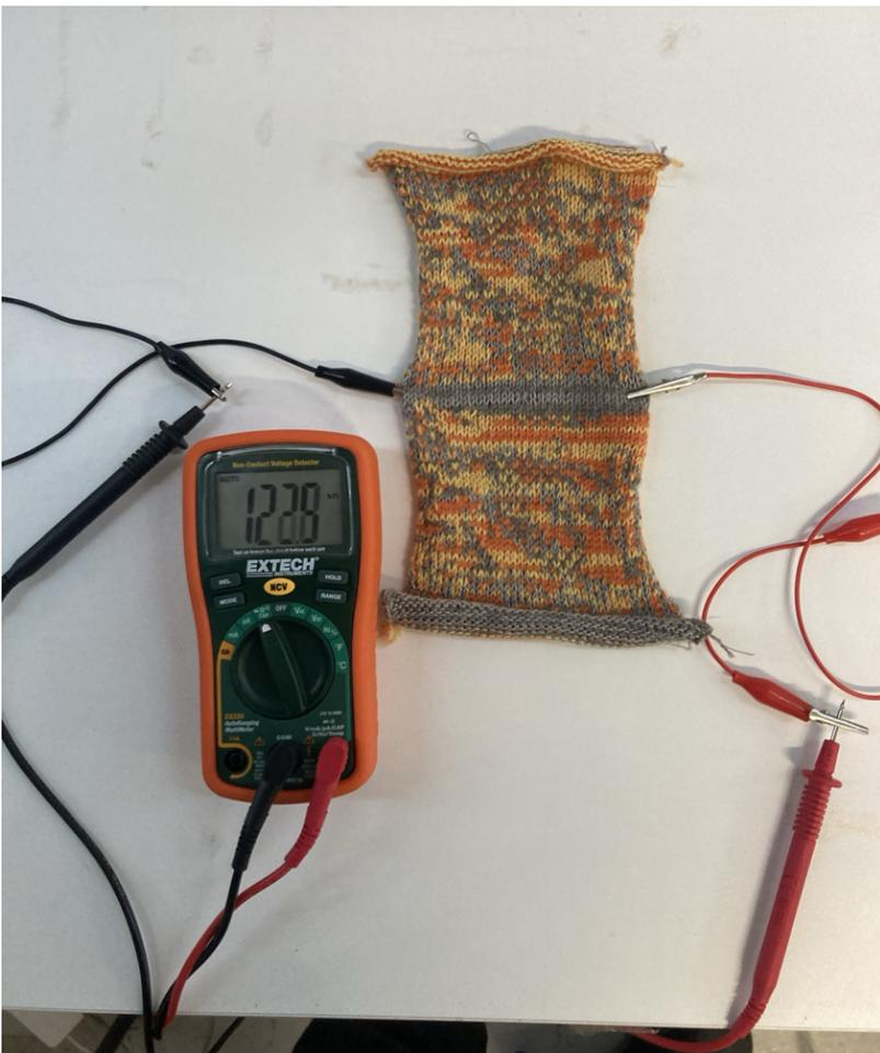
Once the system is connected, you should see a reading of the sample's resistance on the multimeter. Try stretching the sample and the number should decrease! Note that the letters next
