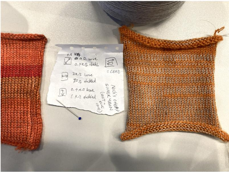
When trialling knit stretch sensors, it's important to know the range of resistances you are working with. You can measure their resistance using a multimeter
