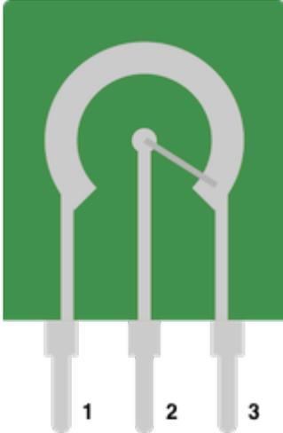
Inside a potentiometer is a large resistive area between pin #1 and #3, the middle pin #2 is called the wiper, and by actuating the pot you can select a position along that resistive area to create a proportional to the voltage between pins #1 and #3.
