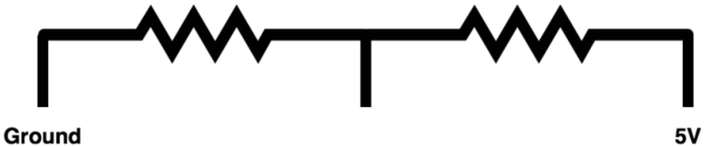
The zig-zag lines indicate resistors, the voltage output we measure with the Arduino comes from this middle point between the two, as the value of the LDR varies it changes the voltage between Ground (0V) and 5V (VCC).
