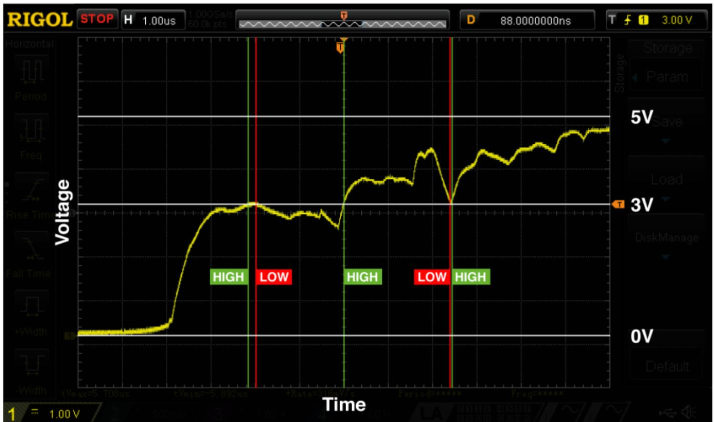
] This diagram shows the signal bouncing up and down over a period of  $10\mu\text{S}$  ( $0.00001$  seconds)
