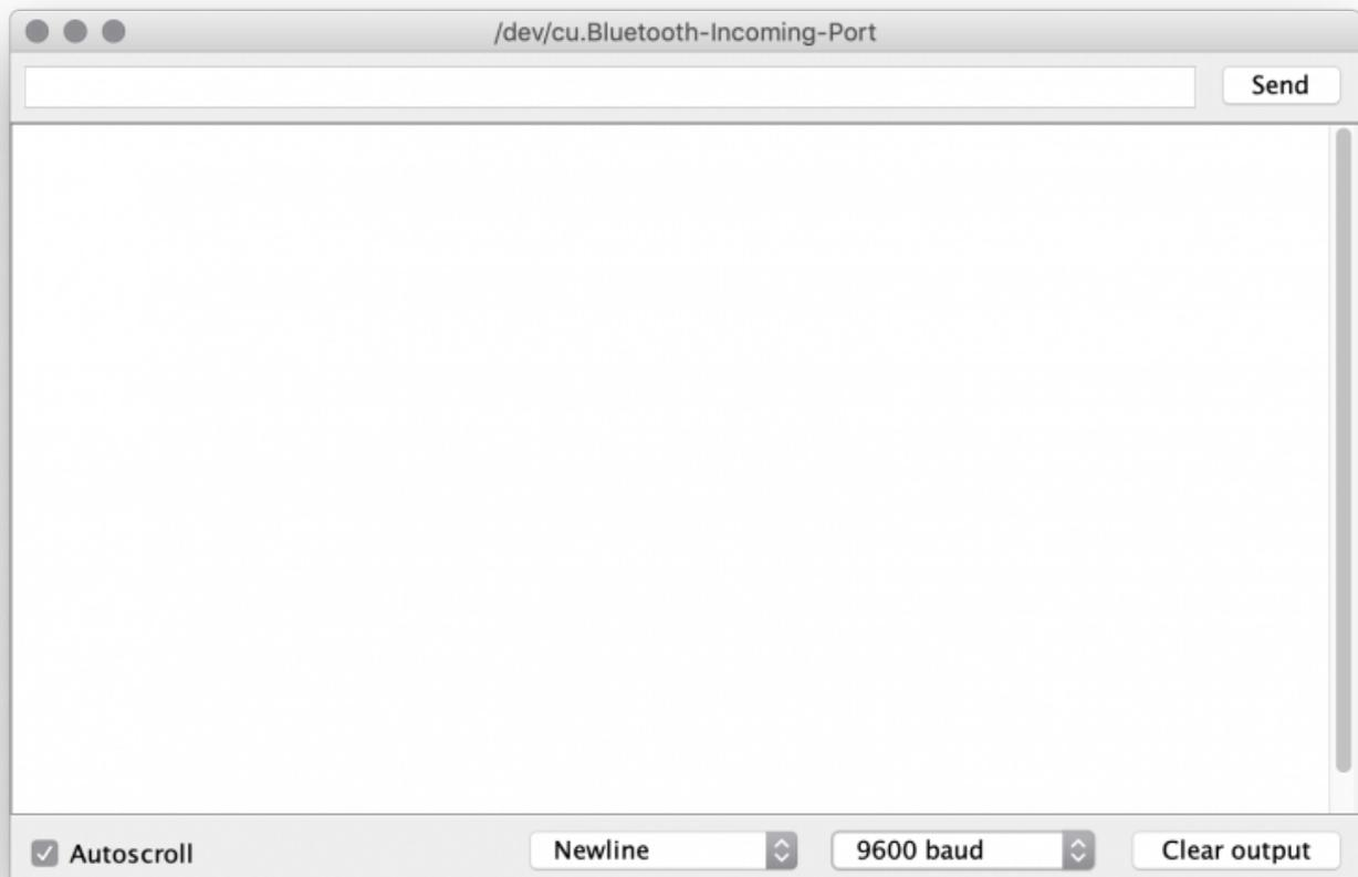
Above is a screenshot of the serial monitor, the first text field is where you can type text and press the send button to transmit to the Arduino. The main window below is where ASCII text will be displayed which the Arduino is transmitting.
