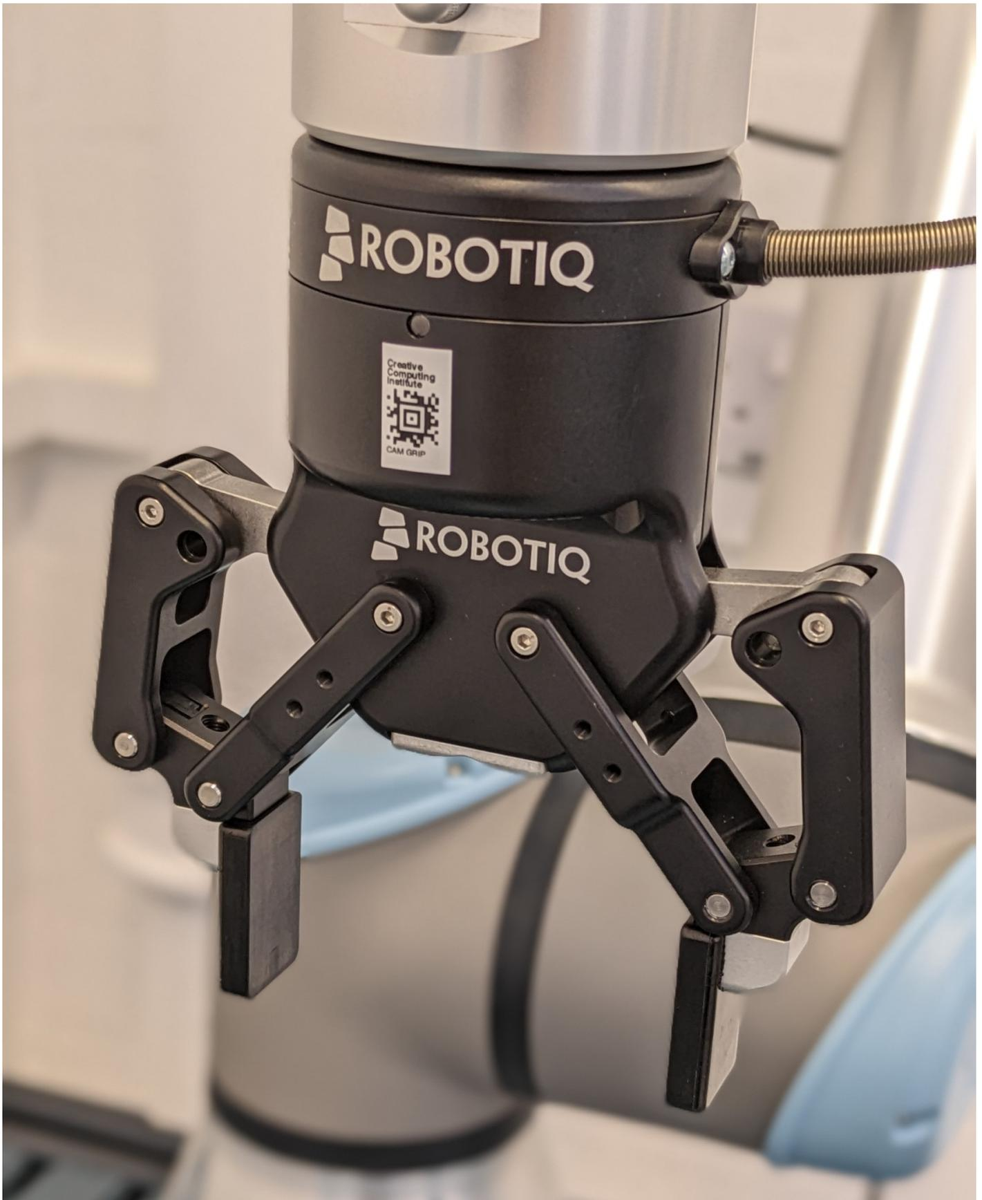
The 2F-85 adaptive gripper by Robotiq is an end-effector that is commonly used with robotic arms such as the UR5e. But the 2F-85 that we have at the robotics lab is rather special as it comes with a camera module as well.
