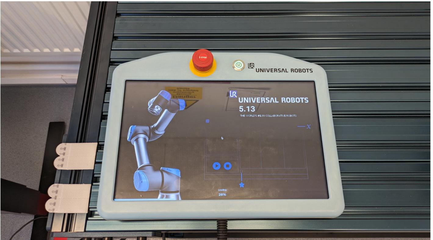
3. Once the loading is complete you will see a getting started screen as shown below. At this stage only the control box has booted up but robot arm itself is not powered on.
