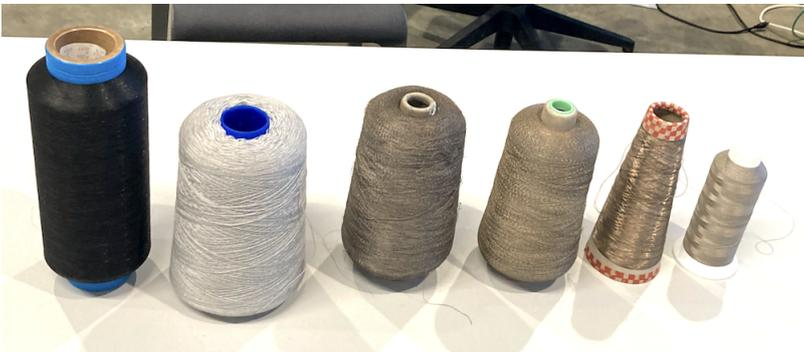
Typically, the conductive yarn is used along with a *carrier yarn*, that adds structural stability, colour, and texture to the knit.
