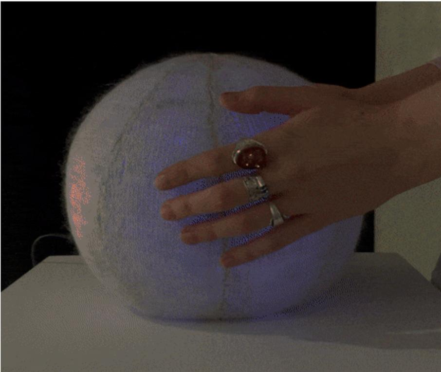
In order to get the sensor to work properly, she both changed the thresholds of the MPR121, and used a set of buffers to smooth the signal.
