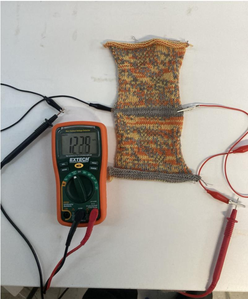
Once the system is connected, you should see a reading of the sample's resistance on the multimeter. Try stretching the sample and the number should decrease! Note that the letters next to  $\Omega$  refer to the magnitude: k stands for 'kilo' ( $\times 1000$ ), and M stands for 'mega' ( $\times 10,000$ ). You want your sample to be at least a few  $k\Omega$  for this to work.
