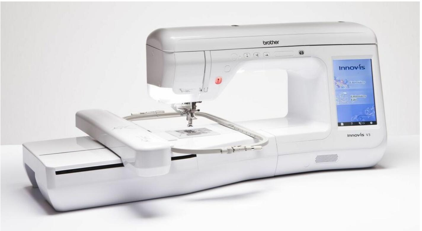
Embroidery machines work by moving a piece of fabric (fixed within a hoop) in the x-y direction, beneath a needle that stitches by moving up and down. In this sense, they have a lot in common with many other 2-axis CAD machines (like laser cutters, routers, plotters), though because of the particular qualities of working with stitches as opposed to straight toolpaths, embroidery software weirdness, and working with different fabrics, there's some practice involved in getting consistent results.
